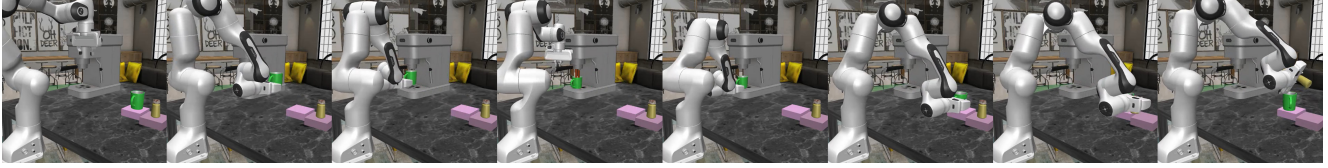
Figure 2. Long horizon task requiring reasoning. This task involves a request for a latte in an interactive scenario. The agent needs to recognize the requirement for coffee with milk and integrate multiple skills, including picking, placing, tool use, pressing, and pouring.
